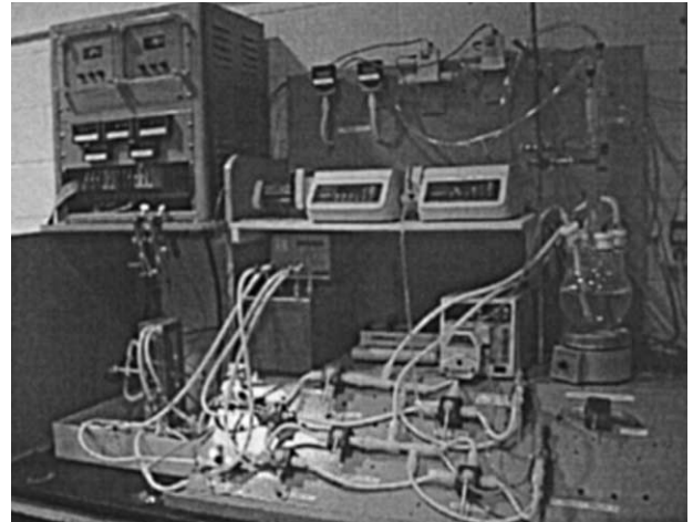
Fig. 1. The dual-flow electrolyte apparatus.
